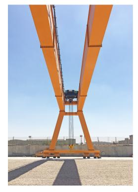
As the ropes of the twin hoist run in opposite directions simultaneously, the load is lifted and lowered without any sideways movement of the hook and can be positioned exactly.
