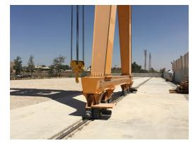
The two portal cranes run on a total of 32 wheel blocks. Eight frequencycontrolled travel drives are used for this.
