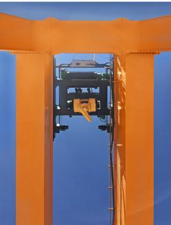
As the ropes of the twin hoist run in opposite directions simultaneously, the load is lifted and lowered without any sideways movement of the hook and can be positioned exactly.
