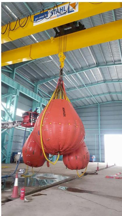
BigBags filled with water were suspended from the crane for the load test.
