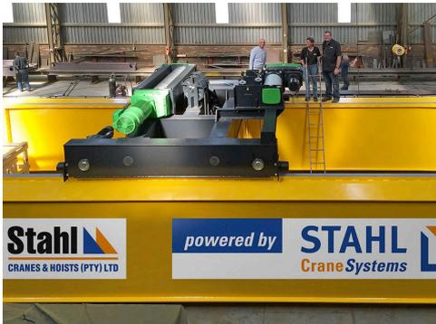
The crane technology from STAHL CraneSystems was first mounted on the beams manufactured by the crane builders Stahl Cranes & Hoist and then tested and shipped to Ghana.
