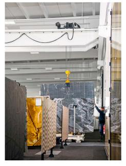
A rail car is used in the overlap area to transport slabs to the adjacent hall.
