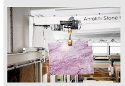
The crane bridge was pulled up on one side – a special solution by Stahl- und Kranbau Oeder.
