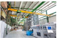
The machining centre in the front section of the building is spanned by a 12.20 metre wide standard crane.
