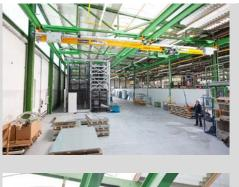
The customised crane in the rear section of the building can be divided. The crane bridge on the right of the photo can then move past the high rack into the front section of the building.
