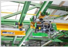
Easy to operate: when the crane operator gives the interlock signal, the control decelerates automatically on approach and interlocks the crane bridges automatically.
