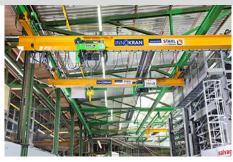
The shorter section of the off-standard crane can travel past the high rack into the front section of the building.
