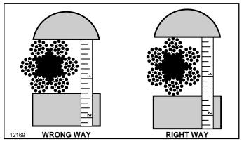
Figure 8-2. Correct Method of Measuring Rope.
