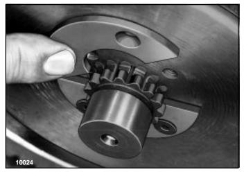
Figure 8-7. Removing Retainer Plates on Load Brake Shaft.
