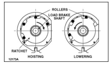
Figure 8-5. Illustration of Roller-Ratchet Brake.
