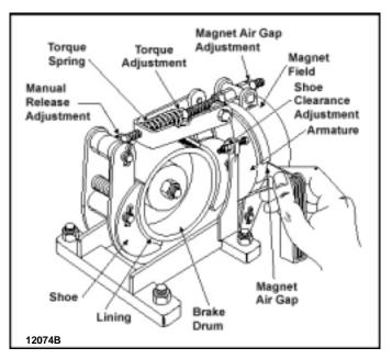
Figure 8-4. Typical Shoe Brake.
