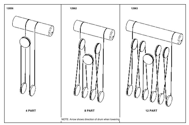
Figure 2-1. Diagrams Illustrating Conventional Type Reeving.
