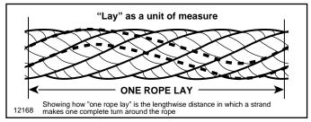
Figure 8-3. Description of One Rope Lay.
