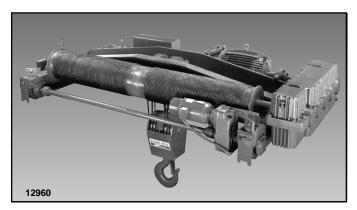
Figure 7-1. Trolley Drive Arrangement.
