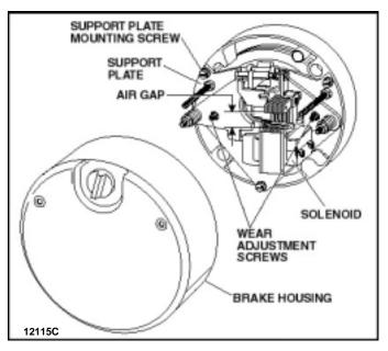
Figure 7-2. Motor Brake.
