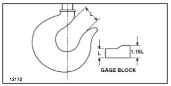
Figure 8-8. Method of Measuring Hook Throat Opening.
