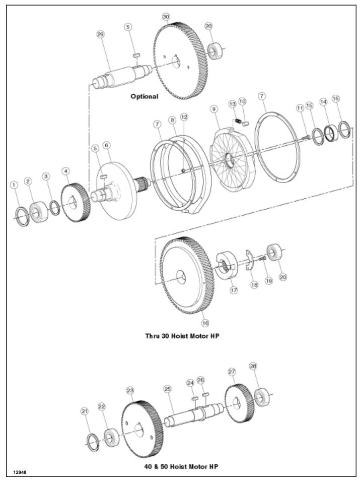
Figure 10-5. Hoist Load Brake Shaft.
