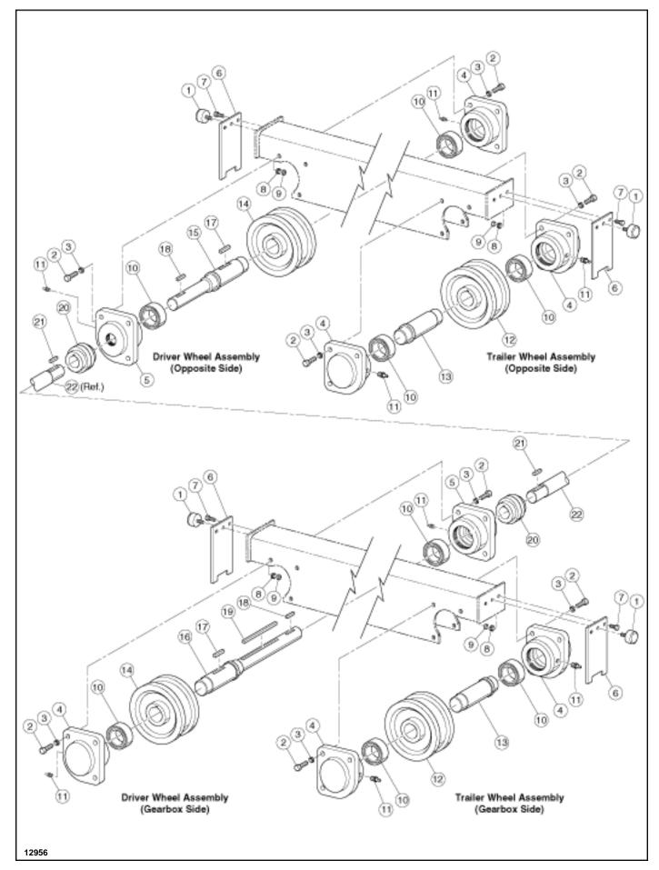
Figure 10-12. Wheel Assemblies and Drive Shaft.
