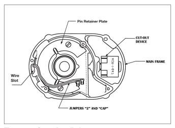
Figure 15 - Stator Installation
