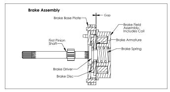
Figure 11 - Brake Field Assembly
