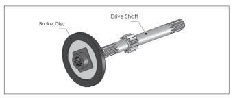
Figure 12 - Drive Shaft Assembly
