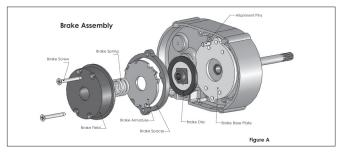
Figure 13 - Brake Assembly
