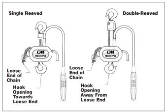
Figure 17 - Chaining Diagram
