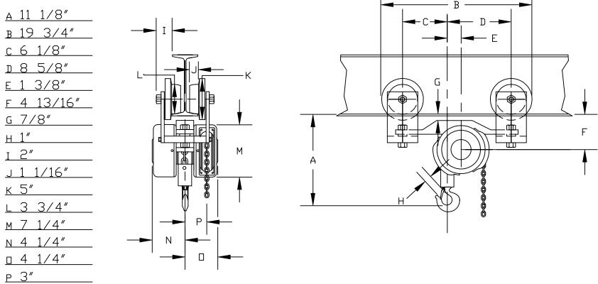
UNIT IS ADJUSTABLE FROM \$5"X10# THROUGH \$10"X25.4# BEAM CUSTOMER MUST TAKE INTO CONSIDERATION FLANGE WIDTH AND THICKNESS. \* DIM. TO WHEEL RUNNING SURFACE
