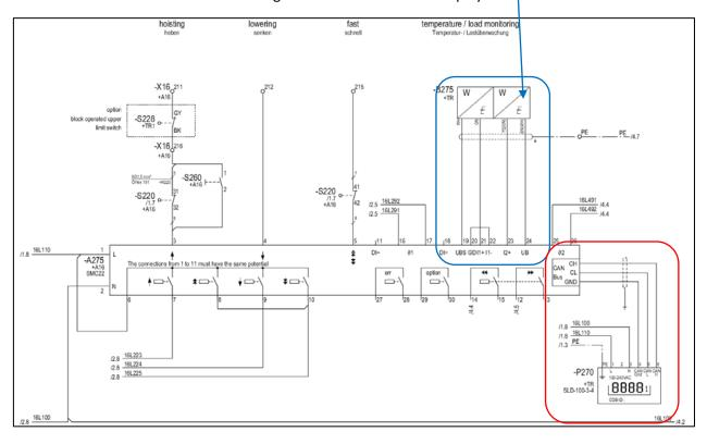
Remove B275 LCP sensor and rewire LCD sensor to SMC22 as shown
