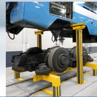
Flexible: underfloor lifting systems make it possible to replace bogies, to work underneath the train and to carry out all kinds of inspection tasks.
