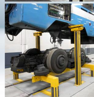
With underfloor lifting systems from Pfaff Verkehrstechnik, maintenance work can be comfortably performed on anything from trams to high-speed trains.
