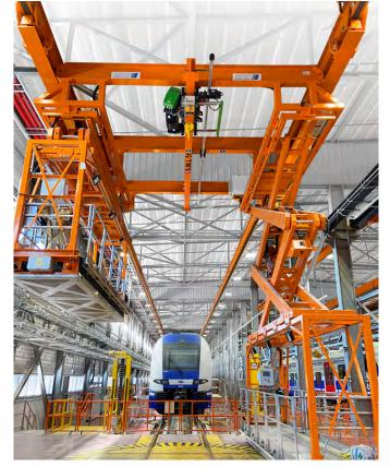
The gap area between the gondola and the train can be completely closed with electric extension modules. When both gondolas are positioned at roof level in paired operation, telescopic railings can be used to create a working area for all-round safe and comfortable work on the roof.
