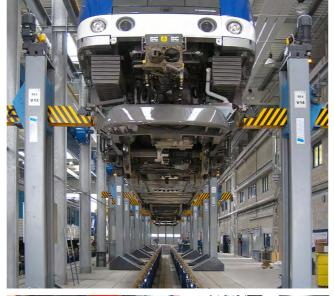
Lifting jack systems are the universal solution for maintenance work on all
