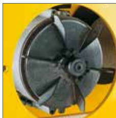
Spring pressure disc brake
