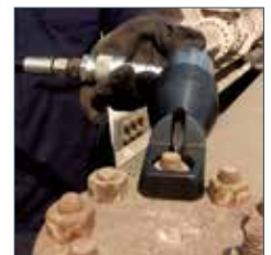
Nut splitters YNS/YNS-AH, SW 11 - 89mm
