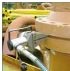
Spreading wedges YSW-14T, 14t
