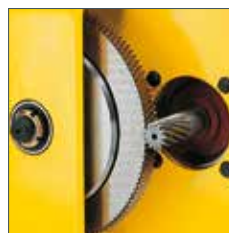
Gearbox with slip clutch
