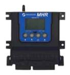
Magnetek's MHR radio controller combines the components of a radio receiver and hydraulic controller into a single unit. When implemented with the MLTX2 bellybox transmitter, it provides a total radio control system for operating the drilling rig. The radio system also manages the RPMs of the rotating drill head and the engine on and off functions.
