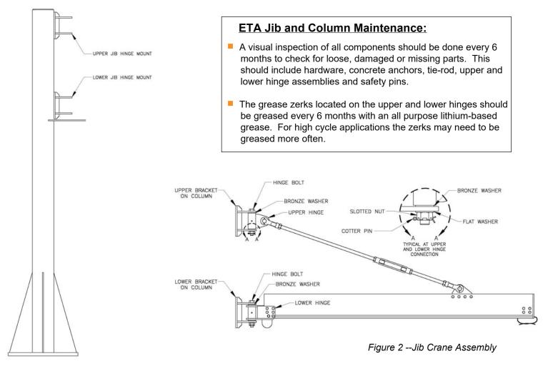
Figure 1 -- Jib Column Assembly
