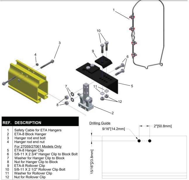
\*Snug tight is the condition that exists when all of the plies in a connection have been pulled into firm contact by the bolts in the joint and all of the bolts in the joint have been tightened sufficiently to prevent the removal of the nuts without the use of a wrench. (RCSC – Specifications for Structural Joints Using High-Strength Bolts Sec. 8.1)
