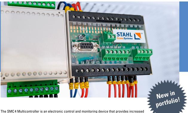
safety for hoists with pole-changing or frequency-controlled drives. By permanently monitoring the condition of the hoist, the SMC4 contributes to safe operation and proper hoist use.
