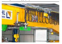
Delivery complete with galvanised C-rail, mounting hardware, cantilever arms for clamping, cable trolley, cables and terminal box
