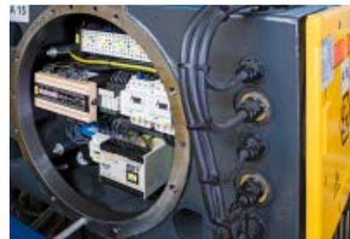
The type of protection for panel boxes for Zone 1, 2 and 21 on cranes and hoists combines types of protection flameproof enclosure »d«, increased safety »e« and protection by housing »tD«.
