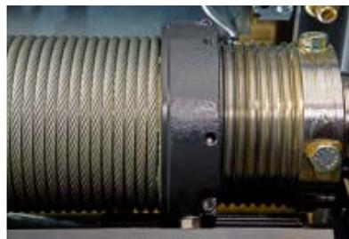
The wear-resistant rope guide in nodular graphite casting GJS (previously designated GGG) is extremely durable and not subject to temperature limitations. The same applies to the chain guide, type of protection used: constructional safety »c«.
