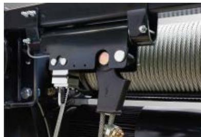
The overload cut-off operates with a dual channel load sensor supplying analog signals. Various sensors are used depending on reeving (LCD, LSD).
