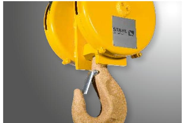
For high and very high travelling speeds the load hook and the solid parts of potential impact surfaces are bronze-coated. In addition, all other exterior surfaces of the bottom hook block can be bronze-coated to prevent sparking.
