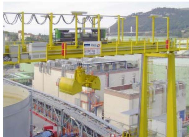
4 Special LNG hoists are used for maintenance work on the pumps of liquid gas tanks. The wire rope hoists have two separately driven rope drums with safe working loads of 2,400 kg. An additional small slewing crane is equipped with an SH 30 Ex wire rope hoist and is used as an auxiliary crane for transporting tools and components onto the tank's platform.
