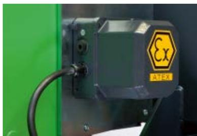
The protection class of the gear limit switch is IP 66. The elements installed are protected by flameproof enclosure »d«, the housing by increased safety »e«.
