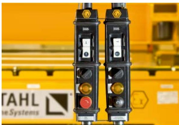
The SWH 5 Ex control pendants are designed specifically for controlling hoists and cranes in hazardous areas. Activation is generally 2-step and permits a quick changeover from 'fast' to 'slow' and vice versa. All control pendants are equipped with an EMERGENCY STOP slam button meeting the requirements of IEC/EN 60947-5-5.
