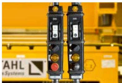
The two-step SWH Ex control pendants in IP 66 protection are used on explosion-protected wire rope hoists for Zone 1.
