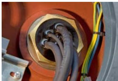
Indirect cable entry, very high safety level from type of protection increased safety »e« and flameproof enclosure »d«. Connection of the Ex e connection box to Ex d by post-type bushing.
