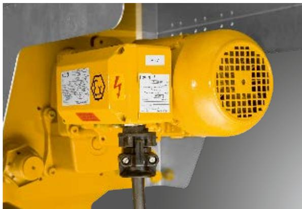
The explosion-protected travel drives Zone 1 and Zone 21 are designed for intermittent operation. They have a sliding rotor motor with conical brake and centrifugal mass for smooth starting and braking characteristics. All motors are pole-changing providing two travel speeds. The particularly quiet gear requires little maintenance thanks to its long-term oil bath lubrication.
