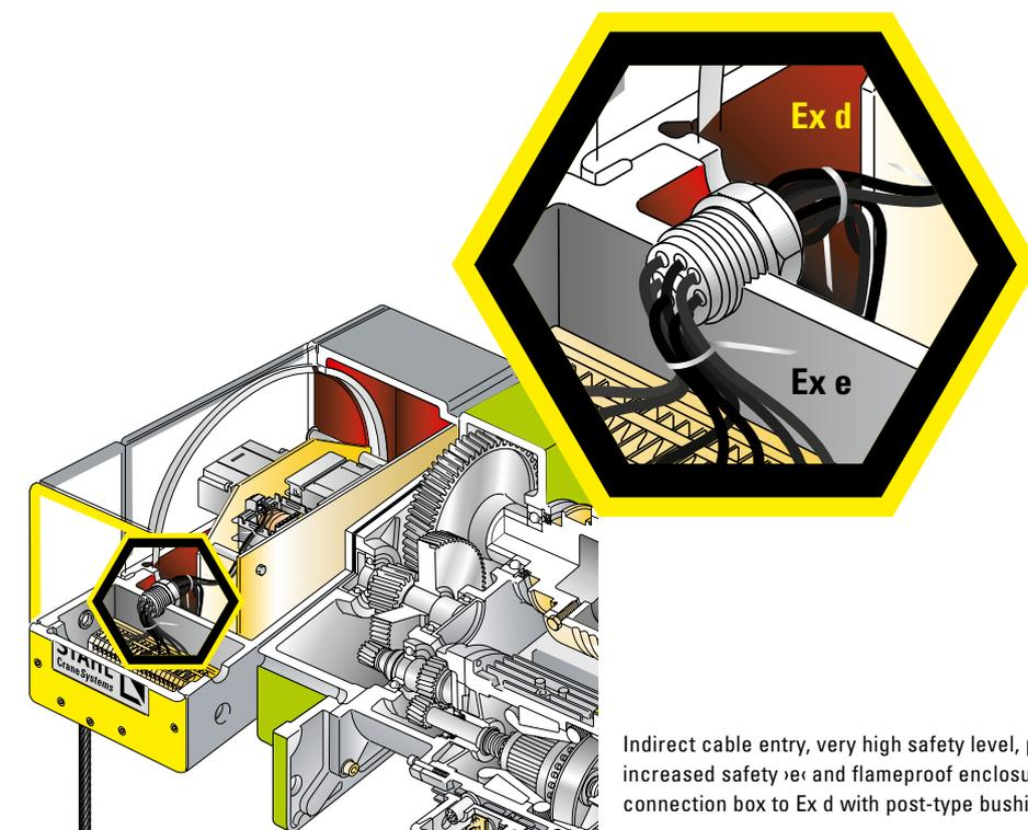
Indirect cable entry, very high safety level, provided by type of protection increased safety »e« and flameproof enclosure »d«. Connection of Ex e connection box to Ex d with post-type bushing.
