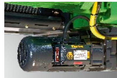
Motors for Zone 1 and 21 are made of grey cast iron, the type of protection combines flameproof enclosure »d«, increased safety »e« and protection by housing »tD«. For Zone 2 the motors are made of aluminium and in type of protection non-sparking equipment »nA«. For Zone 22 the motors are manufactured in IP 66 and protection by housing »tD«.
