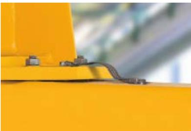
Equipotential bonding is essential for avoiding incendive sparks when installing crane technology in potentially explosive atmospheres.
