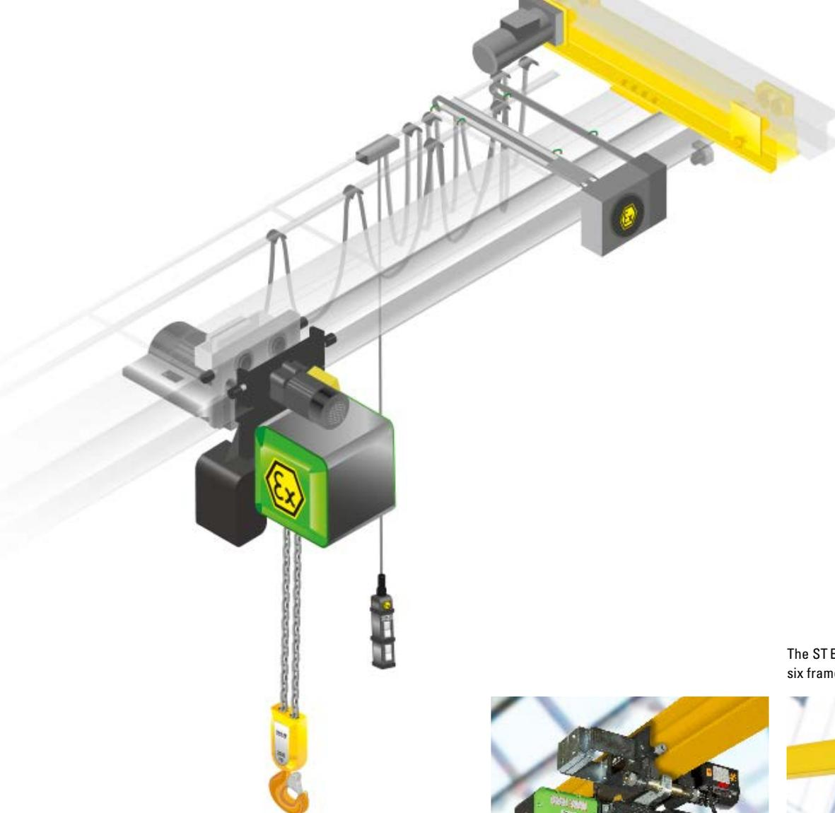
The ST Ex chain hoist for Zone 22 is available in six frame sizes up to a load capacity of 6,300 kg.
