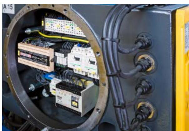
Flameproof enclosure for Zone 1 and Zone 2: the sheet steel or aluminium housings can be used as individual housings or in combination. All components required such as transformers, contactors, fuses, measuring instruments and tripping devices can be installed in the modular-design housing. Post-type bushings provide the connection to the terminal box (in increased safety Ex e).
