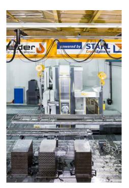
943 mm headroom ... seen from the side, the wire rope hoists completely disappear behind the crane bridge, only the hooks are visible.
