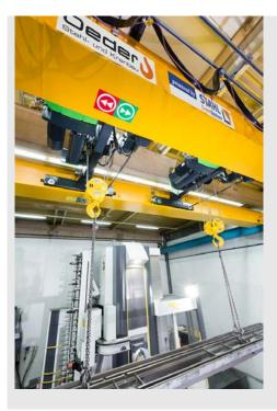
The customised crane is equipped with two SH wire rope hoists each with 8 t S.W.L., which in tandem operation can lift even long loads safely.
