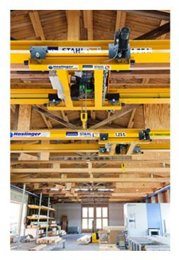
The two double-girder suspension cranes are used for transporting wooden beams and finished wall panels overhead.
