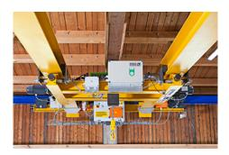
Compact design: the crane's overall headroom is just 57.8 centimetres. Also mounted on the crane: the radio receiver for convenient operation. Conductor lines along the crane bridge are used instead of hampering festoon cables for the power supply.
