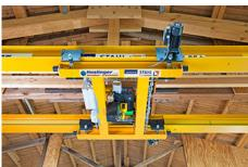
Perfectly adapted to the low-ceilinged wooden structure: only a few centimetres are free between suspension crane and roof beams.
