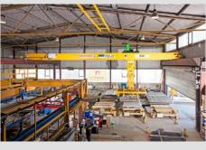
Reinforcements and intelligently limiting the crab's travel made it possible to use the existing crane runway.
