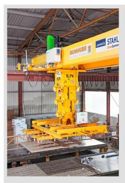
Customised stacker crane from Brunnhuber with components from STAHL CraneSystems: concrete elements weighing up to 5.7 t are lifted from the production line onto transport carts.
