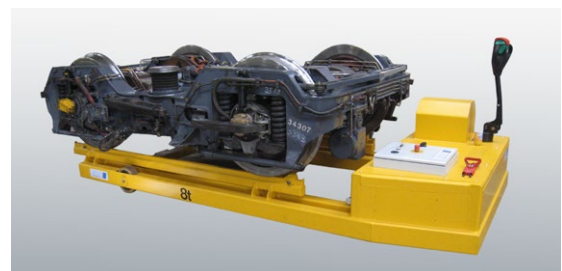
Transport vehicle: moves loads of up to 50 tons.
