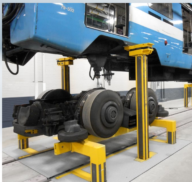
Flexible: underfloor lifting systems make it possible to replace bogies, to work underneath the train and to carry out all kinds of inspection tasks.
