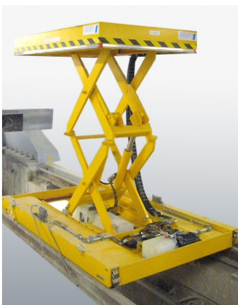
Lifting table: for the removal of bogies, axles and components.
