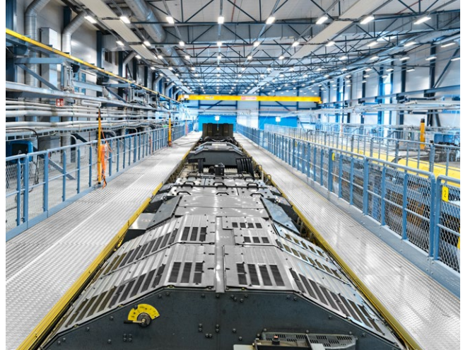
Ergonomic: the roof working platforms provide convenient access to the roof area on all types of vehicles.
