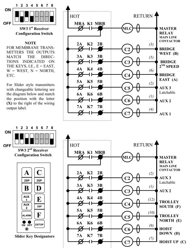
Figure 6-7. 10K9, Two Receivers, Two-Speed East/West Bridge, North/South Trolley and Hoist.
