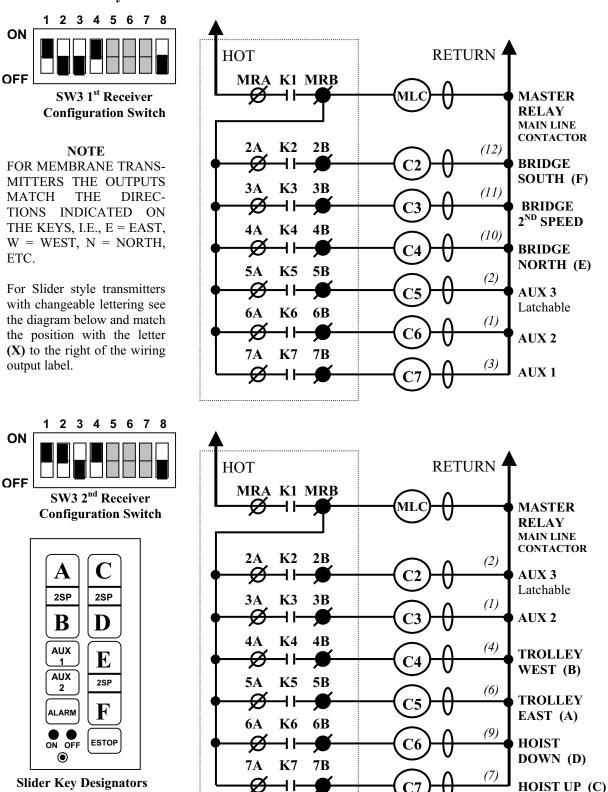
Figure 6-4. 10K9, Two Receivers, Two-Speed North/South Bridge, Single-Speed East/West Trolley and Hoist.
