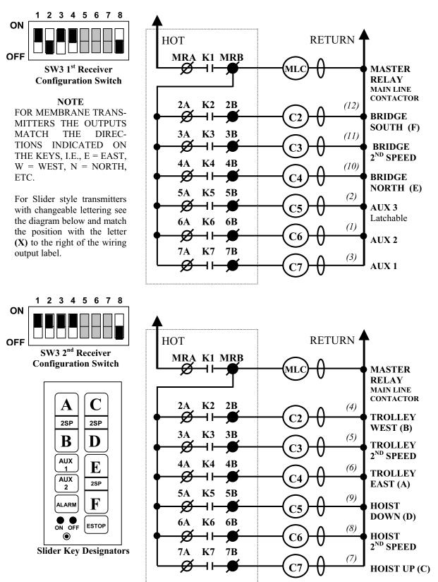
Figure 6-6. 10K9, Two Receivers, Two-Speed East/West Bridge, Single-Speed North/South Trolley and Hoist.
