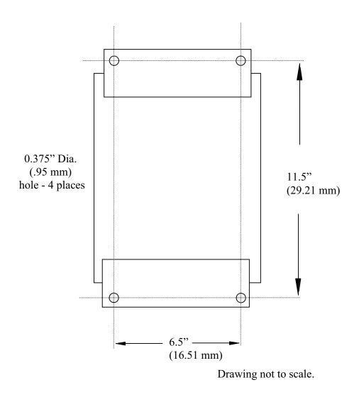
Figure 4-1. Receiver Enclosure Mounting Holes.
