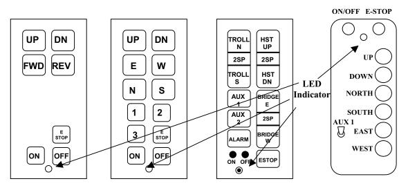
Figure 5-1. Membrane, Slider and Pendant Transmitters.
