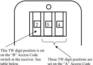
set on the "A" Access Code switch in the receiver. See table below.
