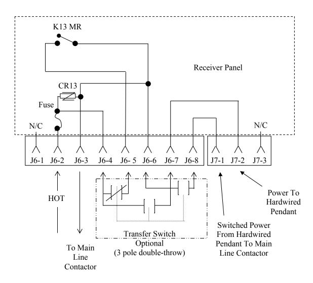
Figure 6-2. Optional Transfer Switch Wiring
