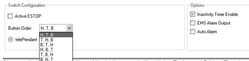
Changes the functional position of the buttons controlling Hoist, Trolley and Bridge. This does not affect Receiver wiring. The Motor controlled by a set button pair will change as "S3-1", "S3-2" and "S3-3" are changed.
