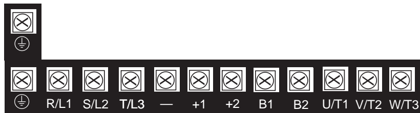
Figure 3-4: Power Circuit Terminal Arrangement
