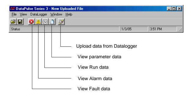
Uploading data stored in the DataLogger is done through the button located on the toolbar or by selecting "DataLogger" and "Upload from the DataLogger" from the Menu. The file must be uploaded before viewing any data. A status bar will indicate the progress of the upload and the history buttons will be highlighted after the upload is complete.
