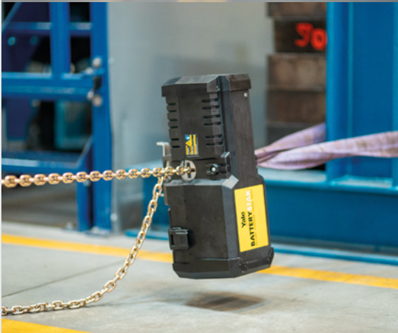
Horizontal pulling by remote control, also in places without power supply.
